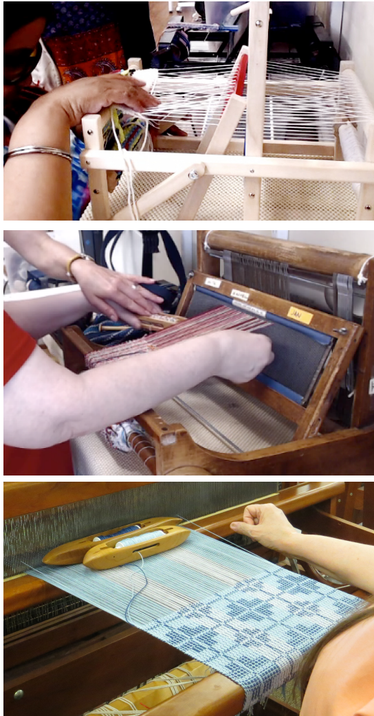
Figure 2: Top: Lisa (weaver) feels tension on the threads to check whether the loom needs to be advanced. Middle: Laura (instructor) provides hand-over-hand support to a weaver while passing the shuttle. Bottom: Amy (weaver) works on a 'summer winter' pattern with two multi-shaded blue yarns.
